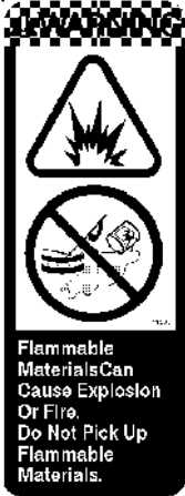
FLAMMABLE SPILLS LABEL - LOCATED ON THE SIDE PANEL OF THE OPERATOR COMPARTMENT.
